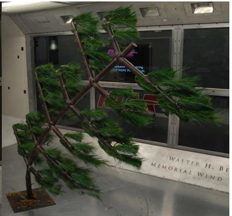
Ehresmann Engineering's pine and custom trees are designed with both antennas and realistic appearance in mind. The branches are RF transparent and UV protected for years of maintenance free tree towers.
