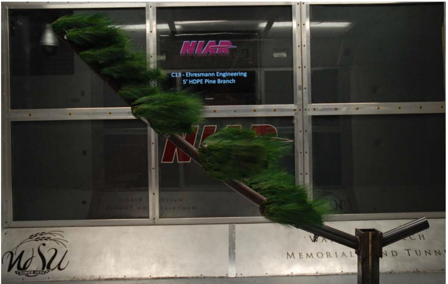
Ehresmann Engineering Inc., is proud to introduce its newly designed Monopine branches for the Communications Industry. Our branches have been wind tunnel tested over **115 MPH sustained wind**. The above 5' branch was tested at **150 MPH sustained wind**. We manufacture the pole and the branches in-house at our 80,000 square facility. This allows us to control the whole manufacturing process. Shipping the monopine with branches can be done at the same time.
